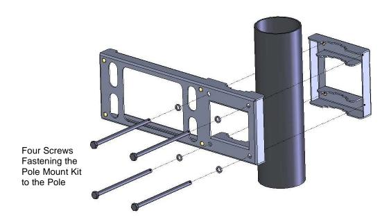
2. Fasten the kit to the pole using the 4 screws, as shown in the photo above.
